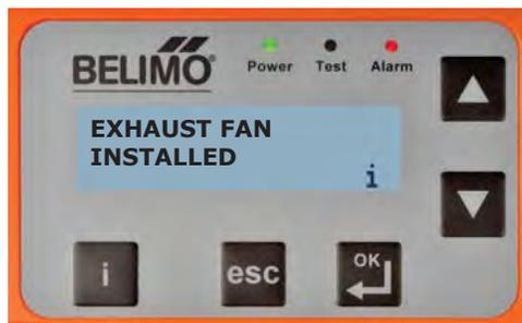
IN THE SETTINGS MENU SCROLL DOWN TO THE DEVICES 1 MENU AND PRESS OK. NEXT SCROLL DOWN TO EXHAUST FAN AND PRESS OK. NOW SET EXHAUST FAN TO INSTALLED USING DN ARROW. THEN PRESS OK. LASTLY PRESS ESC TO GET BACK TO SETTINGS.
