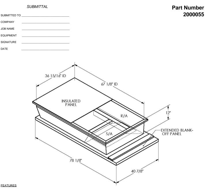
ONE PIECE WELDED CONSTRUCTION
