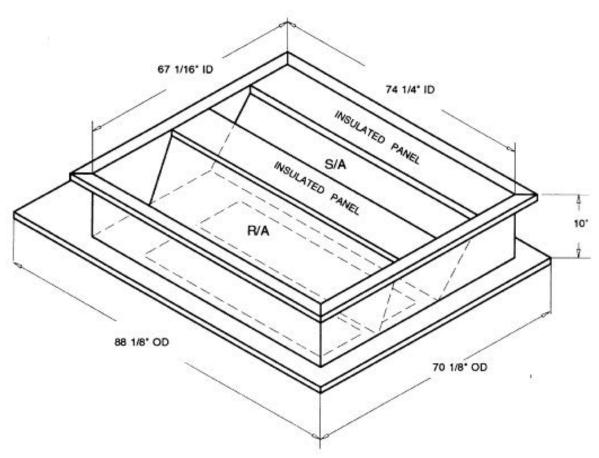
ONE PIECE WELDED CONSTRUCTION
