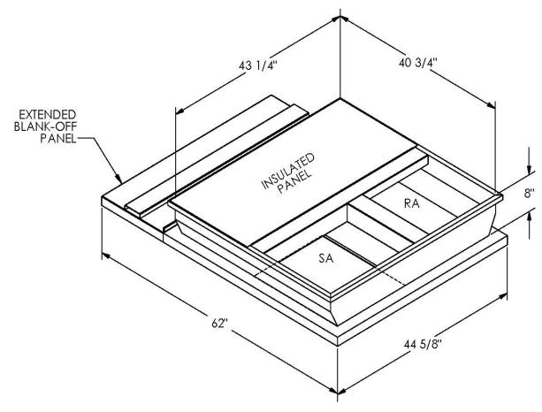
ONE PIECE WELDED CONSTRUCTION
