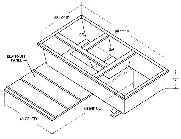
ONE PIECE WELDED CONSTRUCTION
