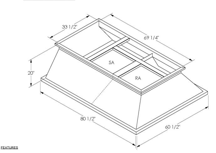
ONE PIECE WELDED CONSTRUCTION
