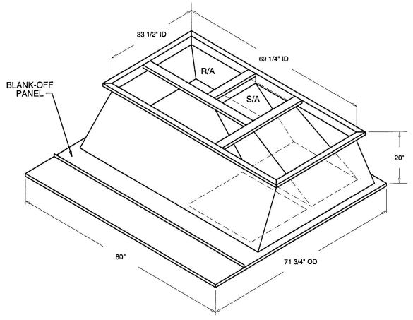
ONE PIECE WELDED CONSTRUCTION
