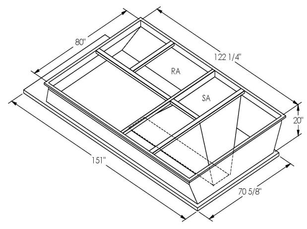
ONE PIECE WELDED CONSTRUCTION
