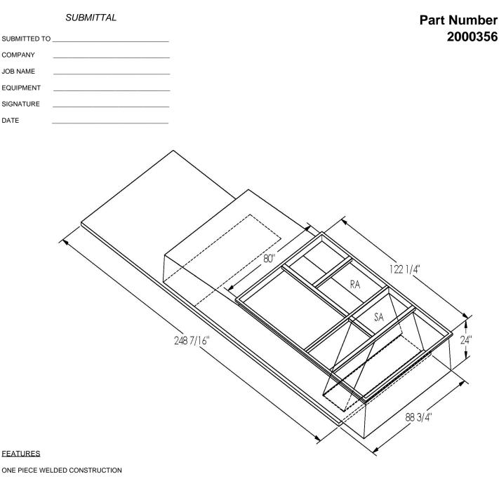
FACTORY INSTALLED SUPPLY TRANSITIONS
