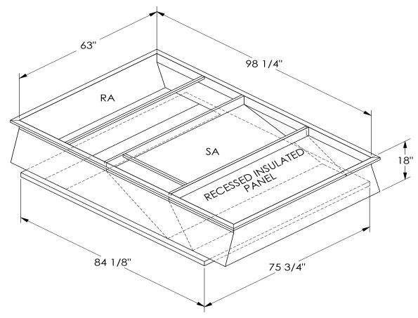
ONE PIECE WELDED CONSTRUCTION
