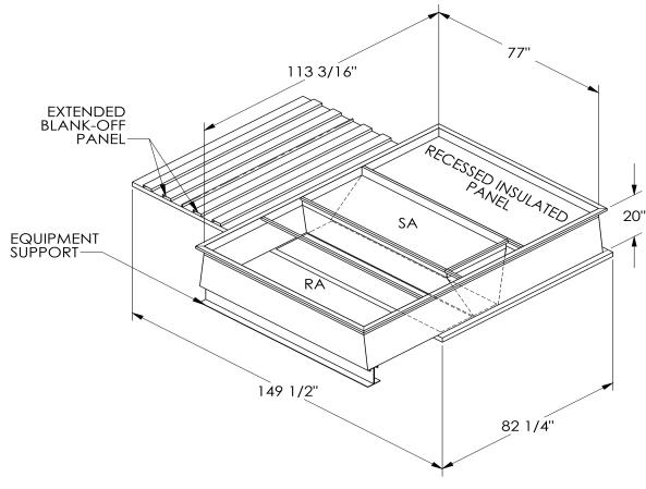
ONE PIECE WELDED CONSTRUCTION
