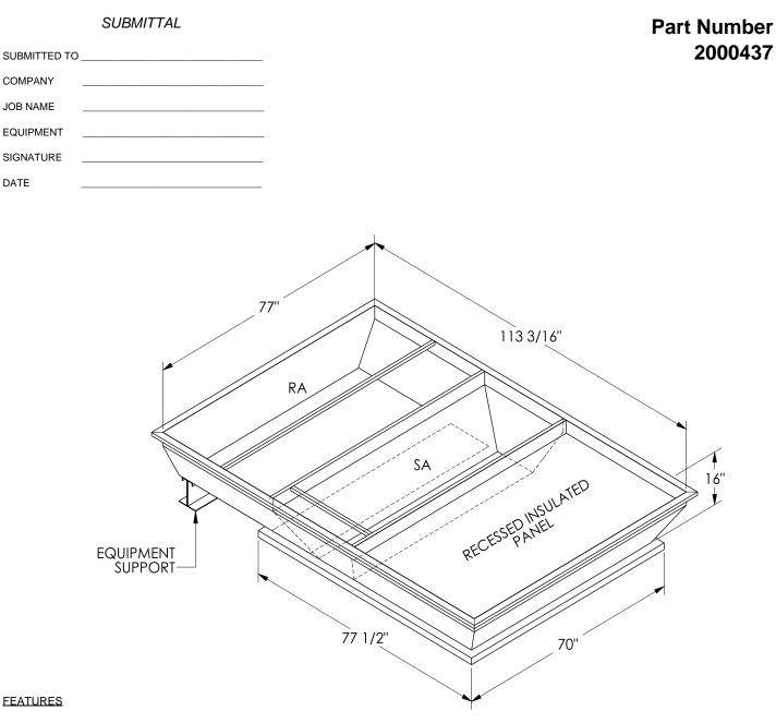
ONE PIECE WELDED CONSTRUCTION
