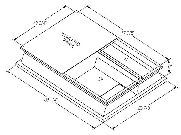
ONE PIECE WELDED CONSTRUCTION
