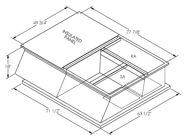
ONE PIECE WELDED CONSTRUCTION
