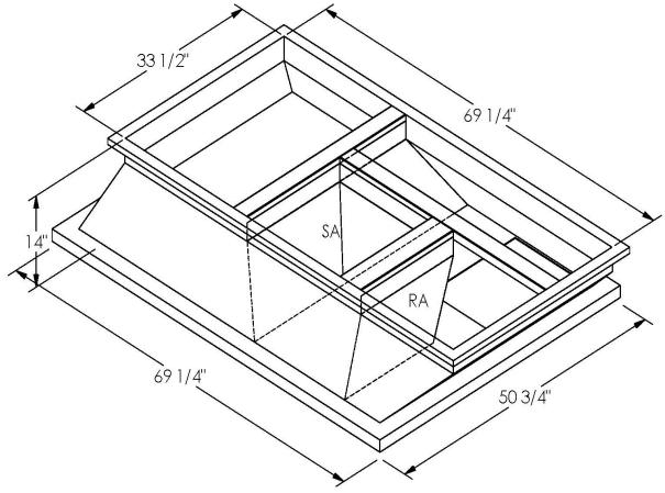
ONE PIECE WELDED CONSTRUCTION
