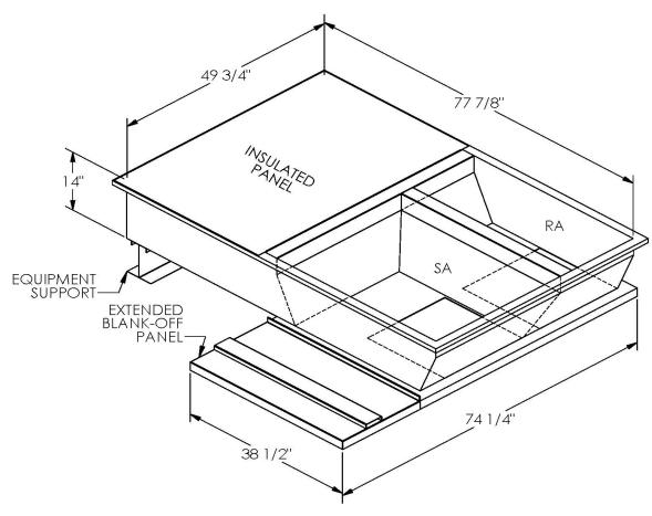
ONE PIECE WELDED CONSTRUCTION
