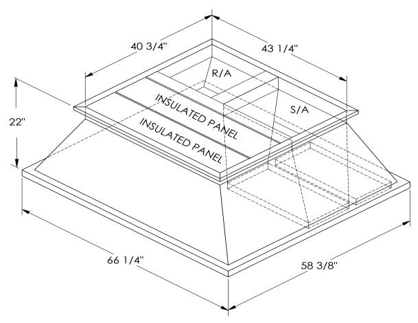
ONE PIECE WELDED CONSTRUCTION
