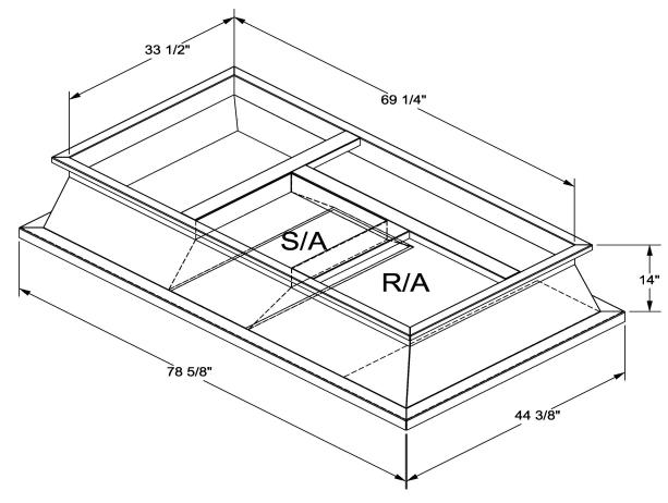
ONE PIECE WELDED CONSTRUCTION
