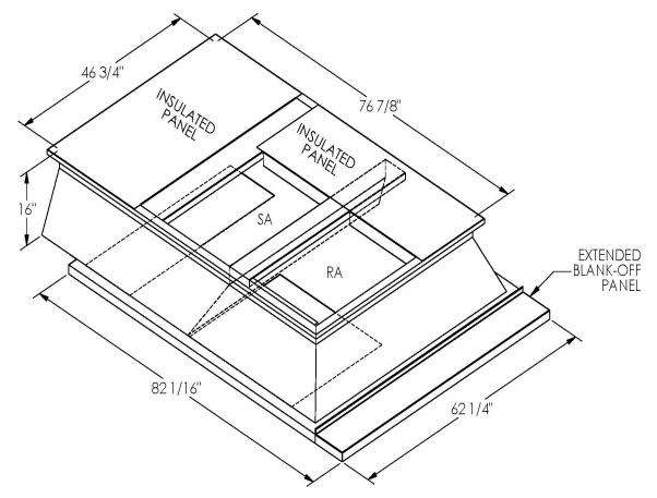
ONE PIECE WELDED CONSTRUCTION
