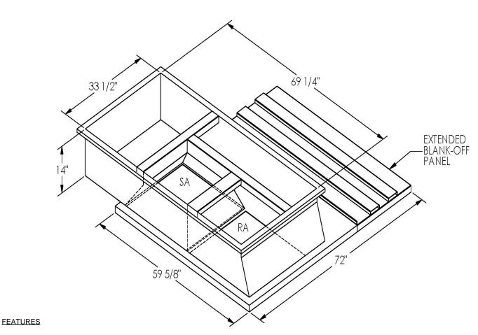
ONE PIECE WELDED CONSTRUCTION
