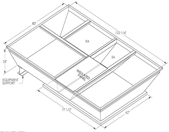
ONE PIECE WELDED CONSTRUCTION
