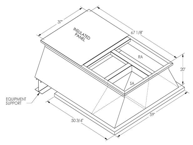
ONE PIECE WELDED CONSTRUCTION
