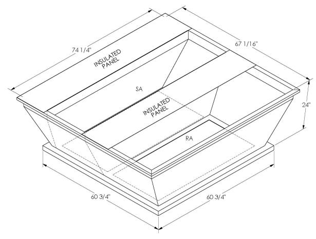
ONE PIECE WELDED CONSTRUCTION
