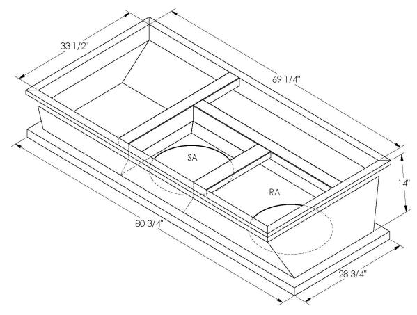
ONE PIECE WELDED CONSTRUCTION
