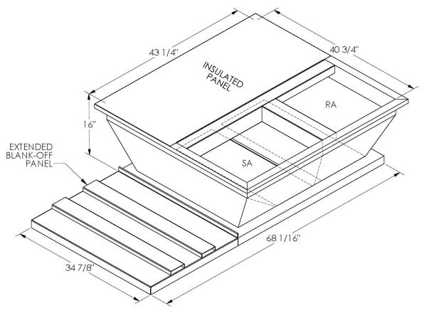
ONE PIECE WELDED CONSTRUCTION
