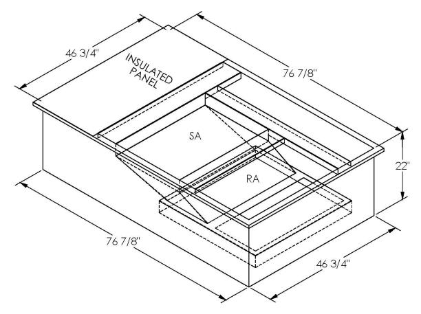
ONE PIECE WELDED CONSTRUCTION
