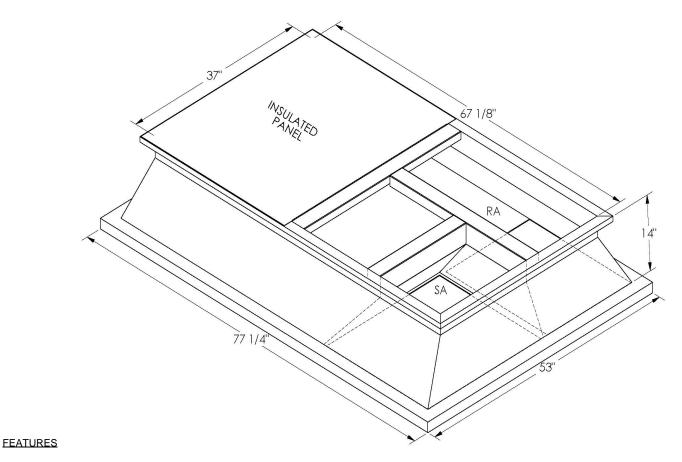
ONE PIECE WELDED CONSTRUCTION
