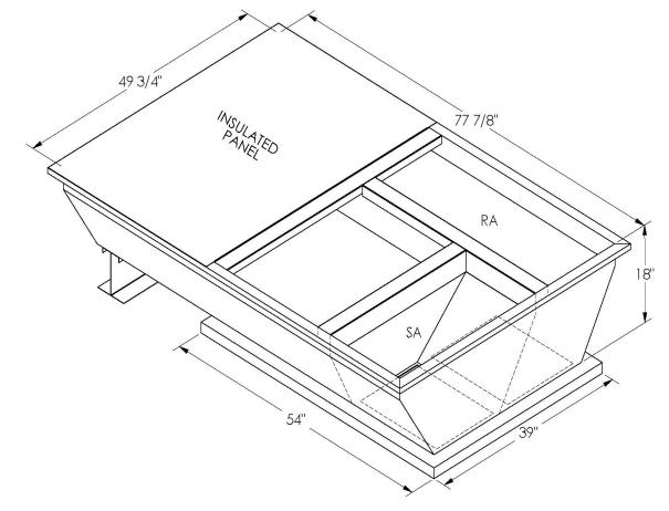
ONE PIECE WELDED CONSTRUCTION
