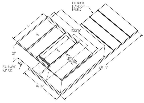
ONE PIECE WELDED CONSTRUCTION
