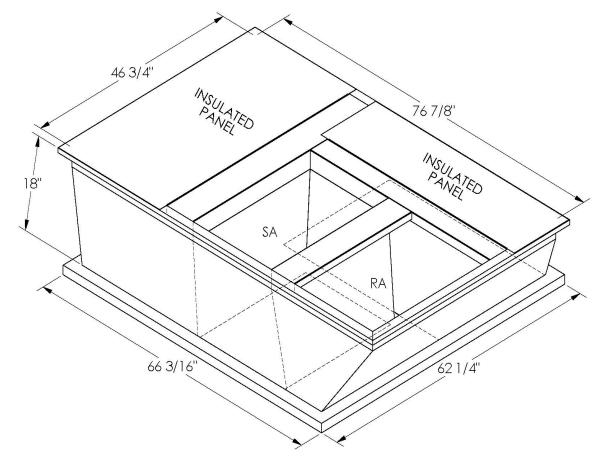
ONE PIECE WELDED CONSTRUCTION
