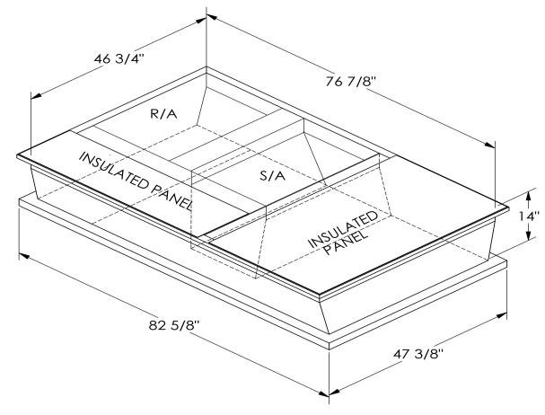
ONE PIECE WELDED CONSTRUCTION
