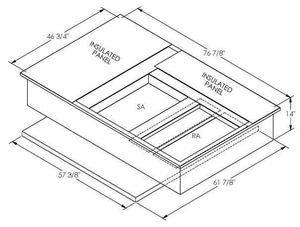
ONE PIECE WELDED CONSTRUCTION
