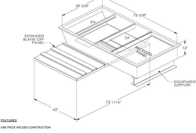
FACTORY INSTALLED SUPPLY TRANSITIONS
