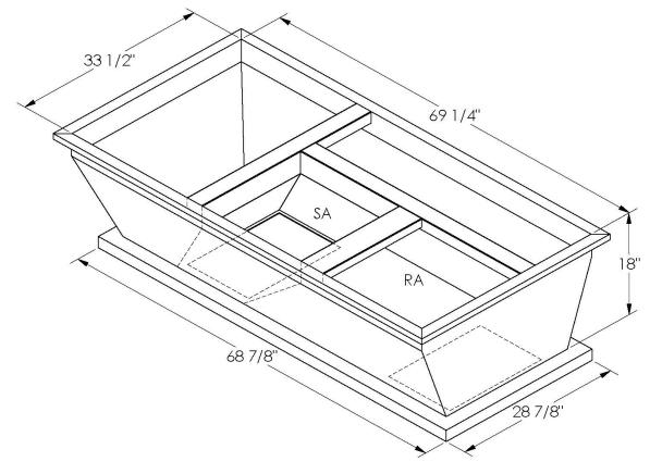
ONE PIECE WELDED CONSTRUCTION
