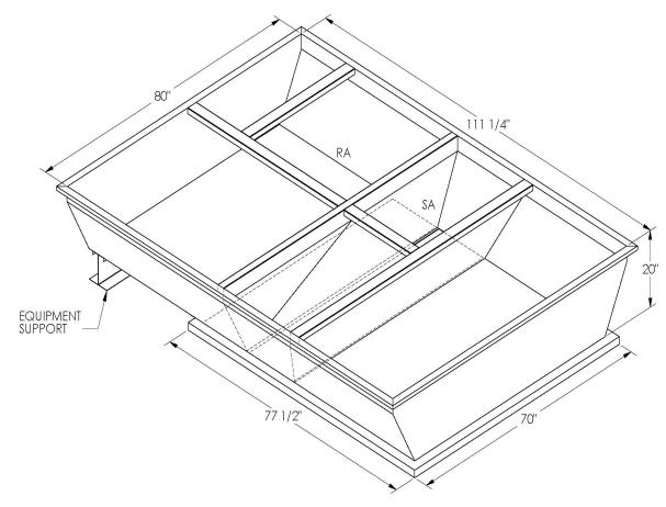
ONE PIECE WELDED CONSTRUCTION
