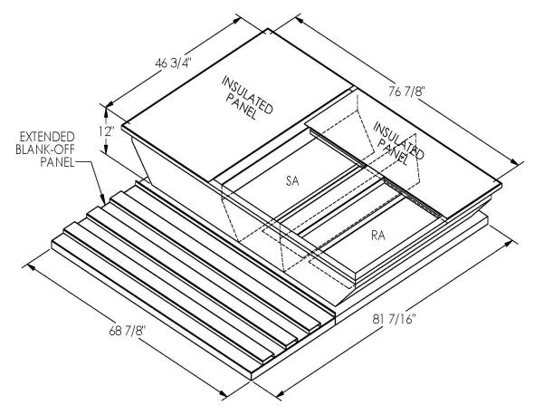
ONE PIECE WELDED CONSTRUCTION
