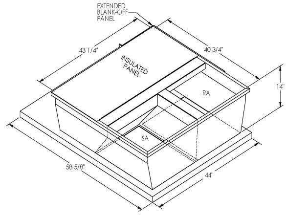
ONE PIECE WELDED CONSTRUCTION
