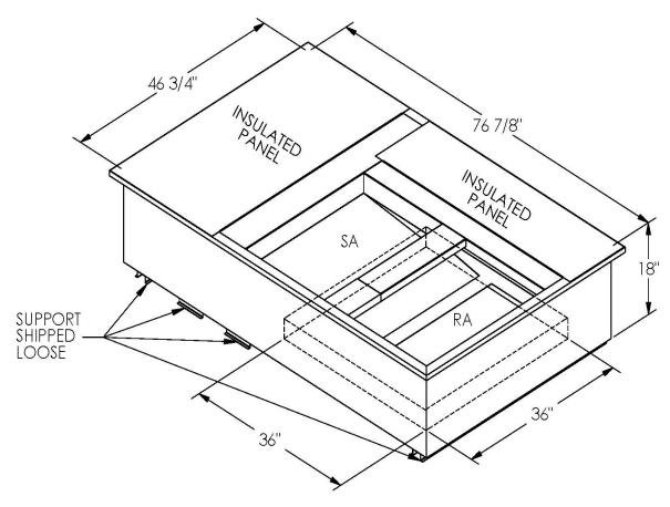
ONE PIECE WELDED CONSTRUCTION
