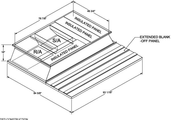
ONE PIECE WELDED CONSTRUCTION
