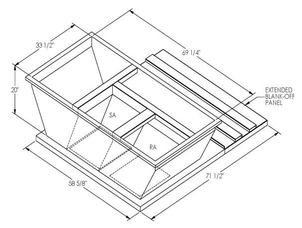
ONE PIECE WELDED CONSTRUCTION
