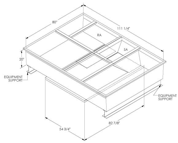
ONE PIECE WELDED CONSTRUCTION
