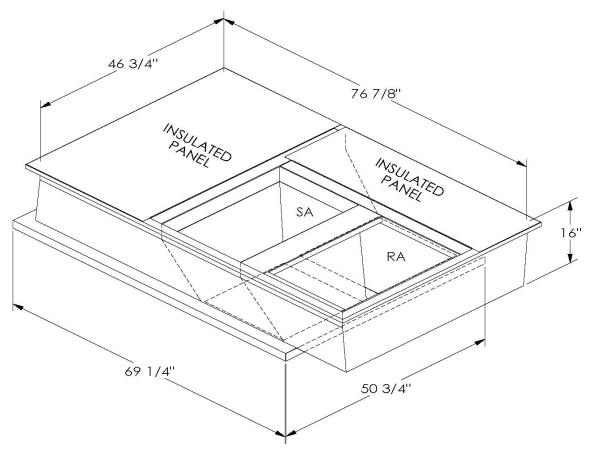
ONE PIECE WELDED CONSTRUCTION
