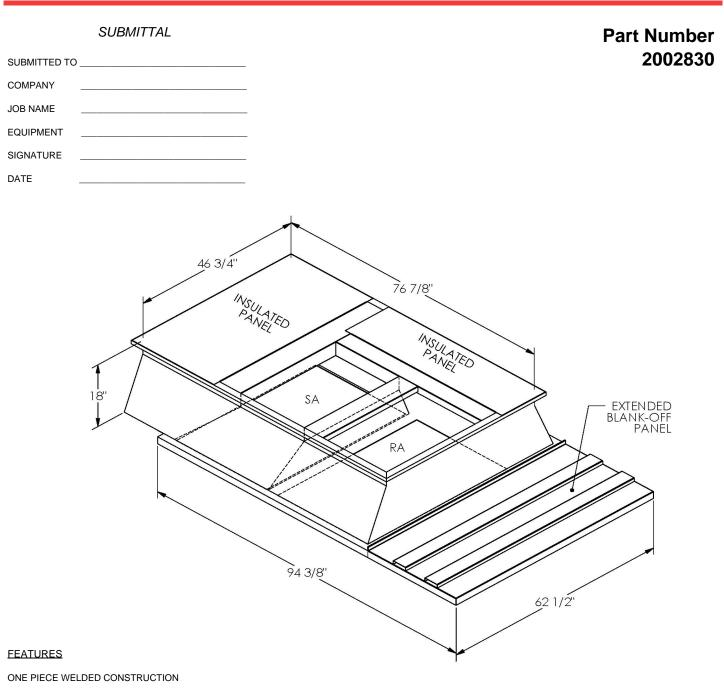
FACTORY INSTALLED SUPPLY TRANSITIONS
