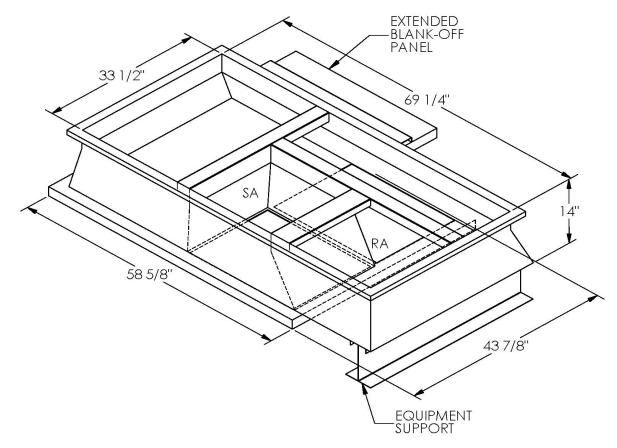
ONE PIECE WELDED CONSTRUCTION
