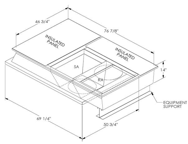
ONE PIECE WELDED CONSTRUCTION
