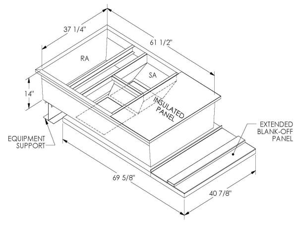
ONE PIECE WELDED CONSTRUCTION
