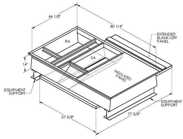
ONE PIECE WELDED CONSTRUCTION
