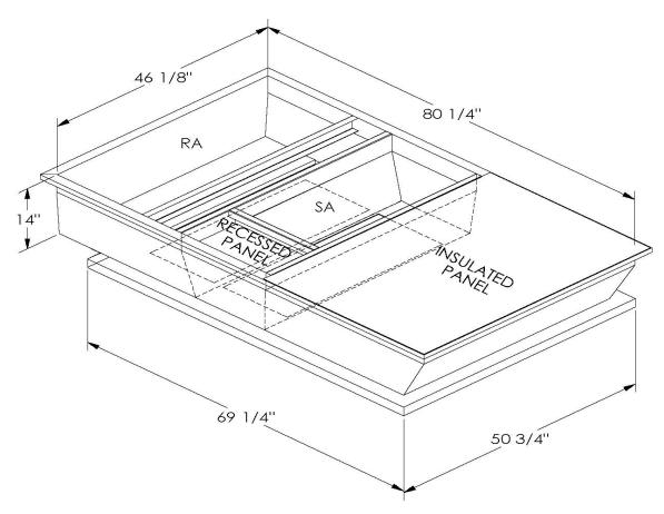
ONE PIECE WELDED CONSTRUCTION
