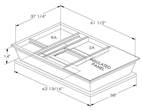
ONE PIECE WELDED CONSTRUCTION
