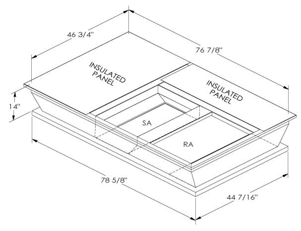
ONE PIECE WELDED CONSTRUCTION
